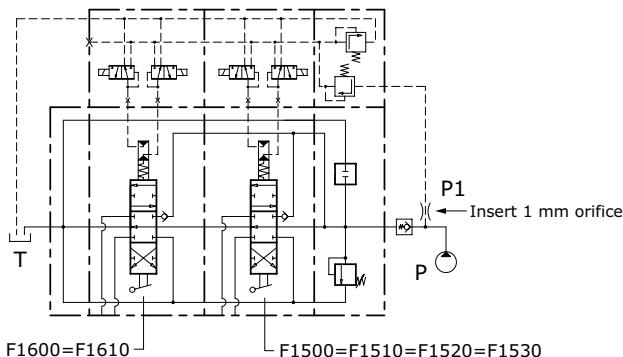
**Electrohydraulic PROPORTIONAL control with fixed pressure reducing valve**
