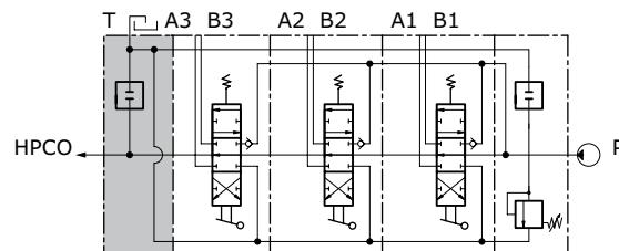
It is possible to transform sectional valve from standard to HPCO version just by ordering the appropriate conic plug:
