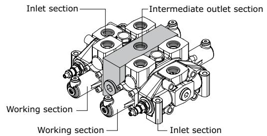
**Complete configuration samples for D12/2 with intermediate outlet section (BG)**
