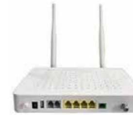
Optical Network Unit
