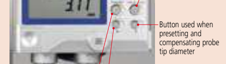
Button used when presetting measuring direction and compensating probe-tip diameter
