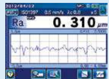
Profile display: One parameter measurement result and the measured profile
