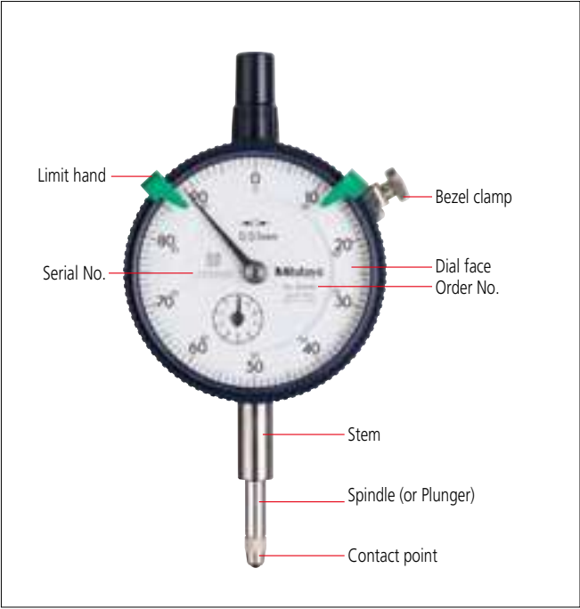
Parts of a dial indicator
