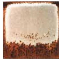
Galvanized steel Z275 (Heavy sign of Rust)
