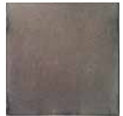
ZINCALUME® steel (No Sign of Rust)
