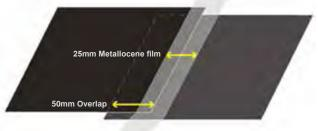
The sections of liner are joined using a heat welding process with a 50mm overlap.
