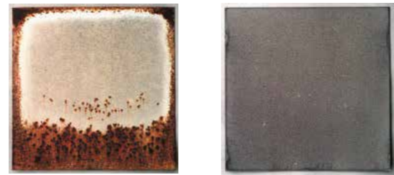
Galvanised steel Z275 (Heavy sign of Rust) ZINCALUME® steel (No Sign of Rust)
