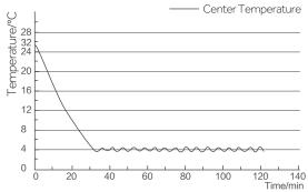
Refrigerating speed under no load condition at 25°C ambient temperature
