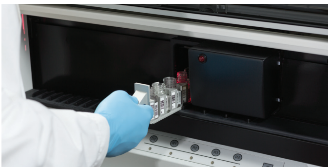
Onboard barcode reader allows real-time reagent management.
